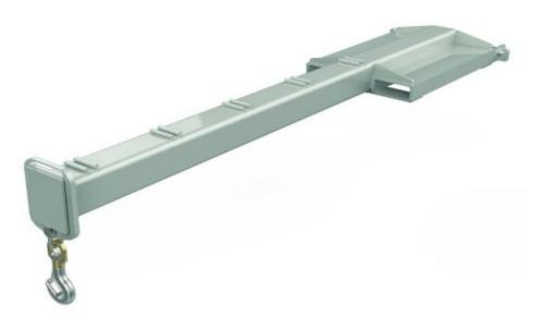
Note: All lift truck attachments affect the safe working load of a lift truck. End users should consult their lift truck supplier to ensure the lift truck is rated for use with these attachments. In the case of a slung load when lifting a jib attachment, the net lifting capacity should be 0.8 times the rating of the lift truck to allow for the swinging load. Please consult your local lift truck supplier for rating.
